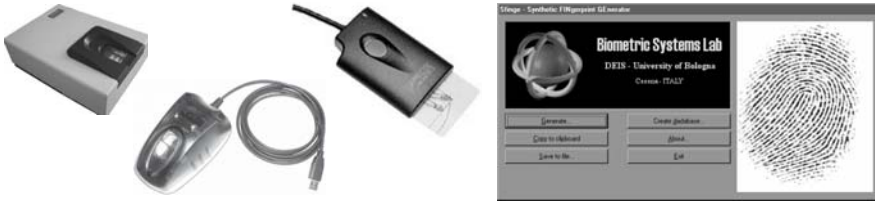
Figure 6.13 From left to right: the three sensors used for collecting DB1, DB2 and DB3, respectively, and a snapshot of the tool which generated synthetic fingerprints in DB4.
