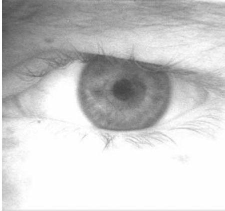
Figure 3.5 Captured iris image. An example iris image as captured by the Wildes et al. passive sensor is shown. Notice that this initial stage of sensing captures not only the iris but also surrounding portions of the eye region. Subsequent processing must more precisely localize the iris per se . R. Wildes, Iris recognition: an emerging biometric technology. Proceedings of the IEEE , 85 (9), 1348–1363, 1997 (© 1997 IEEE)
