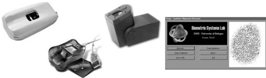
Figure 6.1 Fingerprint database generation. From left to right: the three sensors used for collecting DB1, DB2, DB3, respectively, and a snapshot of the tool which generated synthetic fingerprints in DB4.
